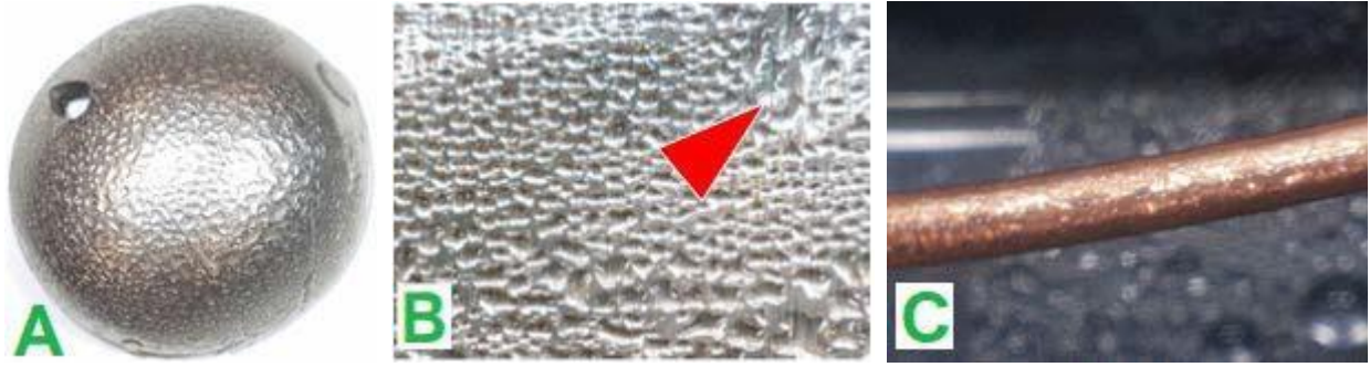
Fig. 5. Micrographs of water droplets in various stages of formation on the bumps and spikes.
