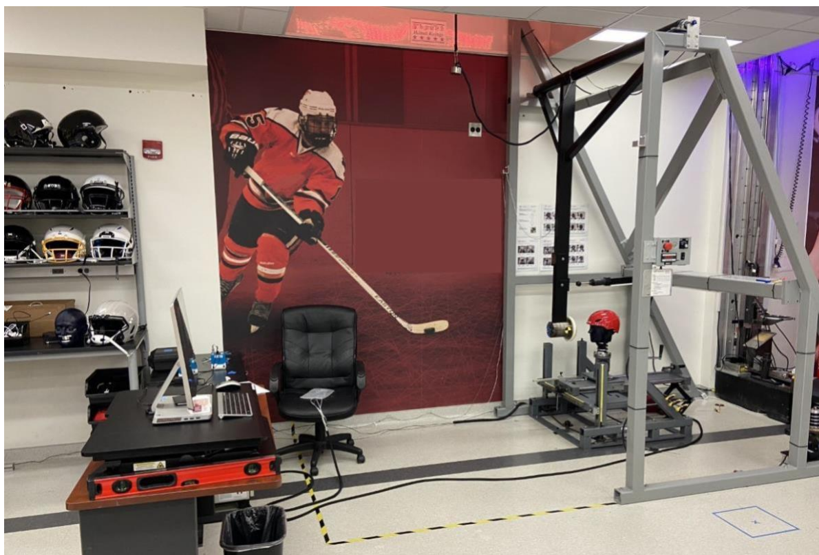
Figure 2: The front impact condition is shown on the right with the pendulum system.
